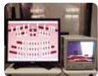
Camera automatically points to whichever speaker the operator selects on the computer
